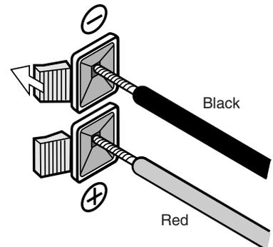
While holding the button of each speaker terminal, insert a conductor of the connection cord.
