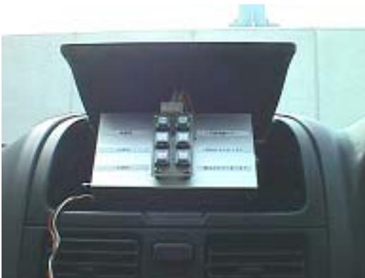
Three buttons that allowed the driver to input 'no change', 'weak', or 'strong' sleepiness were on the top panel of a recording device.
