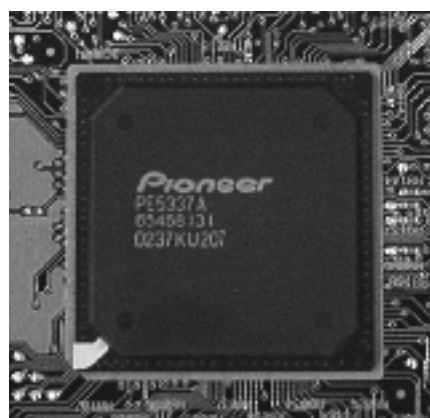
図2 Stream Processor LSI(PE5337A)の外観
